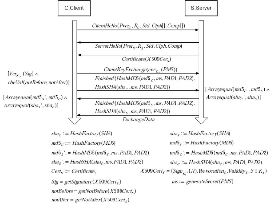
Figure 3: The cryptographic protocol implemented in SSLSocket.java
